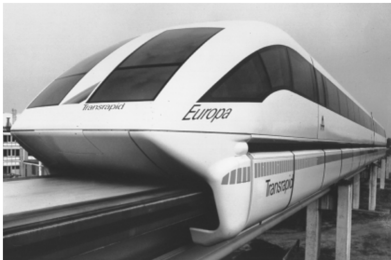
Fig. 32 Experimental magnetic levitation (Mag-Lev) train in development in Europe and Japan, employ bodies with 6061 and 6063 structural members.
