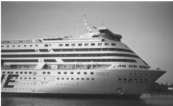
Fig. 19 The superstructure of many ocean liners, ferries, and most naval ships is of welded 5xxx alloy construction, providing lightweight and excellent corrosion resistance.
