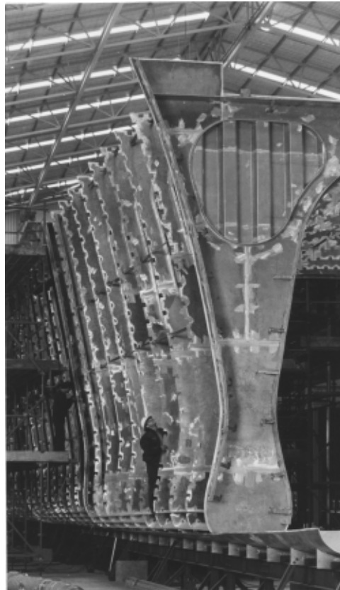
Fig. 17 Single- or multiple-hull high-speed ferries employ several aluminum-magnesium alloys—5083, 5383, and 5454—as sheet and plate (along with 6xxx extruded shapes) with all-welded construction.
