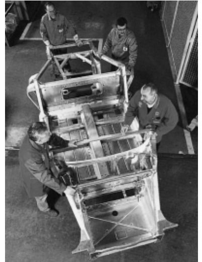
Fig. 22 Automotive structures are likely to employ increasing amounts of 5754-O formed sheet for parts such as internal door stiffeners or the entire body-in-white.
