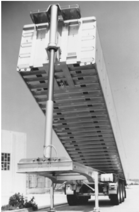
Fig. 7 Heavy dump and tank trucks and trailer trucks may employ 2xxx extrusions for their structural members.
