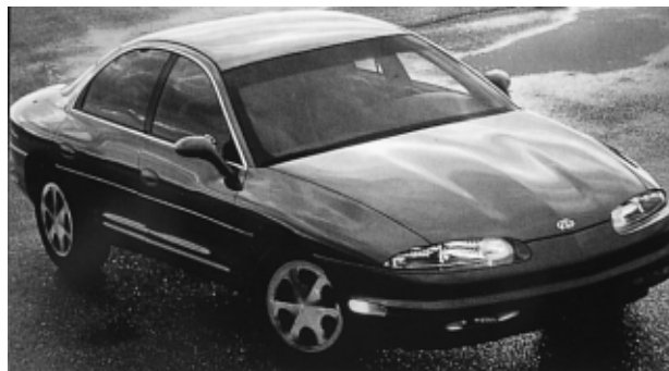
Fig. 36 The General Motors Aurora, like many other production automobiles, has aluminum closure panels of alloy 6111-T4.
