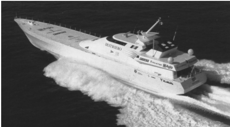
Fig. 15 High-speed, single-hull ships such as the Destriero, employ 5083-H113/H321 machined plate for hulls, hull stiffeners, decking, and superstructure.
