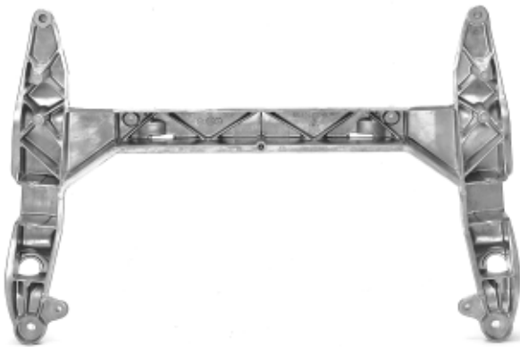
Fig. 41 Aircraft components are made from high-strength cast aluminum alloys, such as alloy 201.0.
