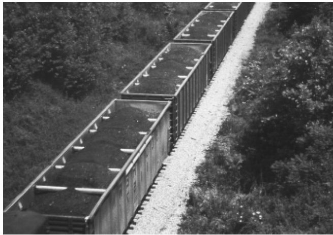
Fig. 20 Rugged coal cars are provided by welded 5454 alloy plate construction.
