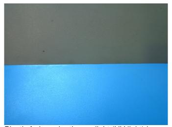
Plastic fade under the sunlight (UV light) is a common issue in appliances exposed to the elements. It's been battledÂÂ for years and chemical additives have been developed to aid this issue. Image to the left represents two <u>injection mould</u> ingÂÂ plastic samples. Bottom blue part was stored away from sunlight, top sample is the same material but was subject to the sunlight for 36 months. Sample contained maximum amount of UV stabiliser.
