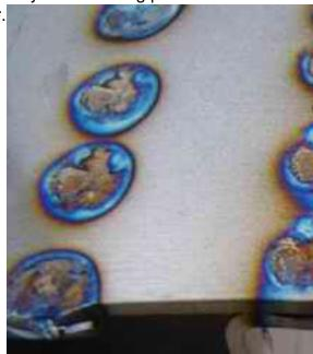
It is a great high speed process to attach two sheets of metal together. The drawback of spotwelding is that it significantly effected welding area. This is a problem in some applications as designers have to hide welding spots via edge bending of <u>stamped metal parts</u> or by covering it.
